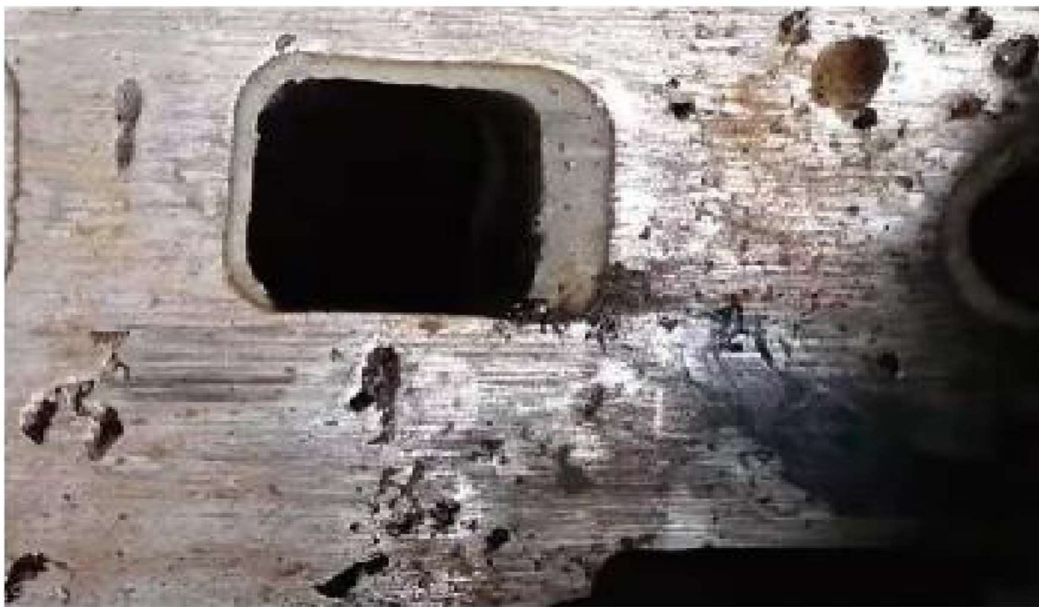
FIG 4: Carbon slag, sand hole, porosity defects are founded in large numbers at the same time.
