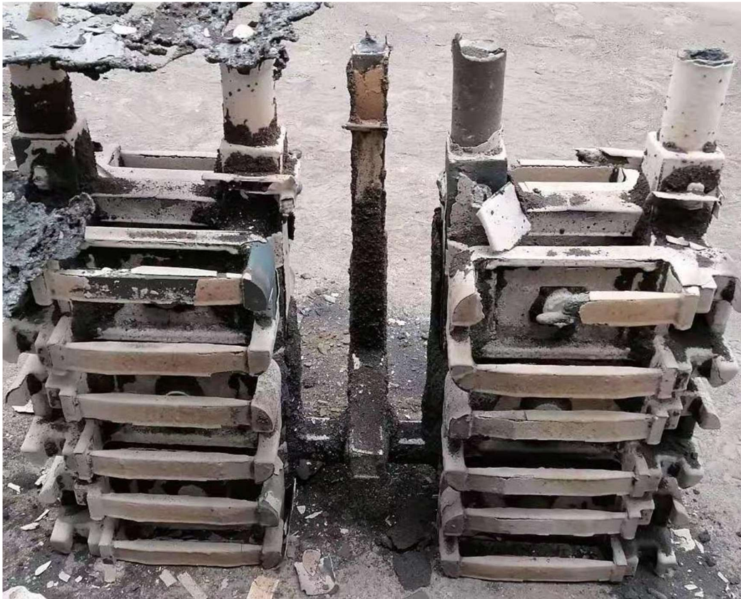
FG. 17: Burn pattern before pouring(casting result)
