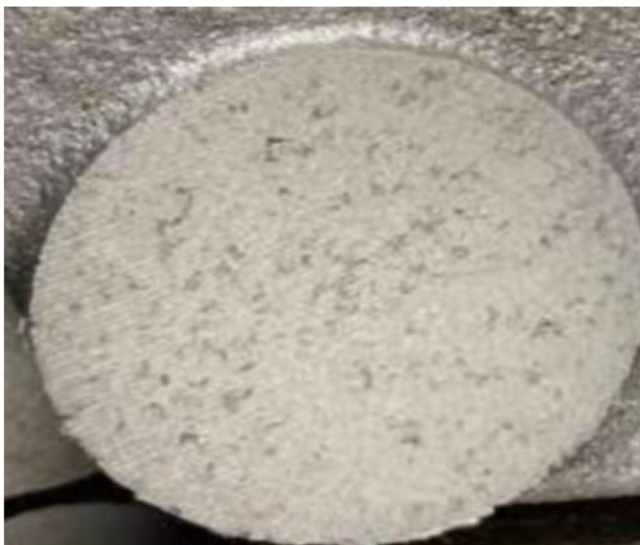
FIG. 2: Internal carbon defect due to vanishing of white pattern
