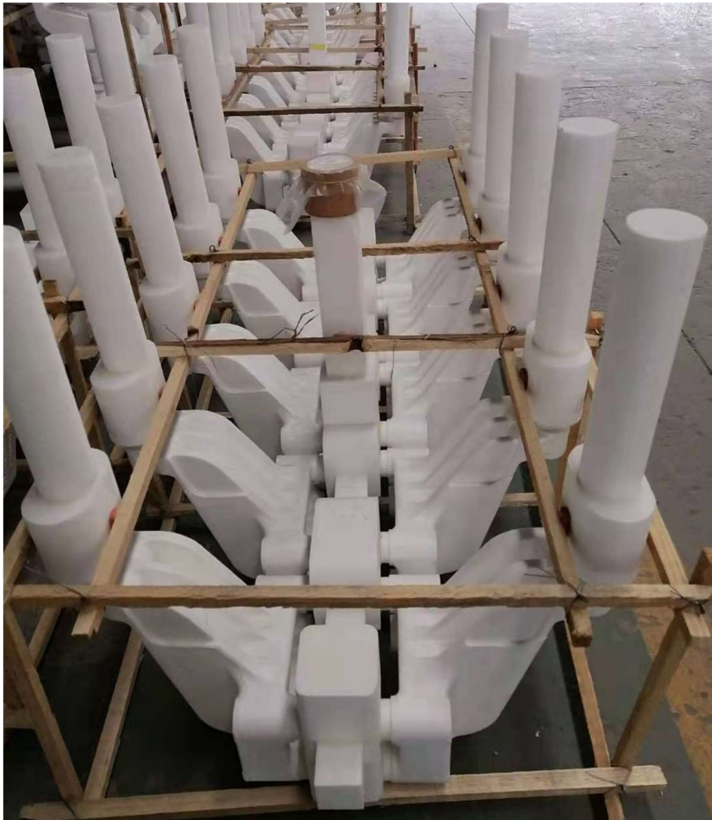
Attached Figure 15: Firing before pouring process
