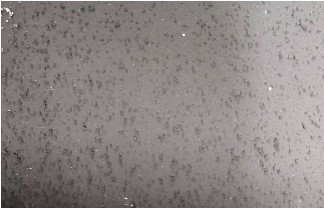
FIG 5: The continuous carbon slag layer formed on the inner surface of the coating of the ERP white pattern after combustion
